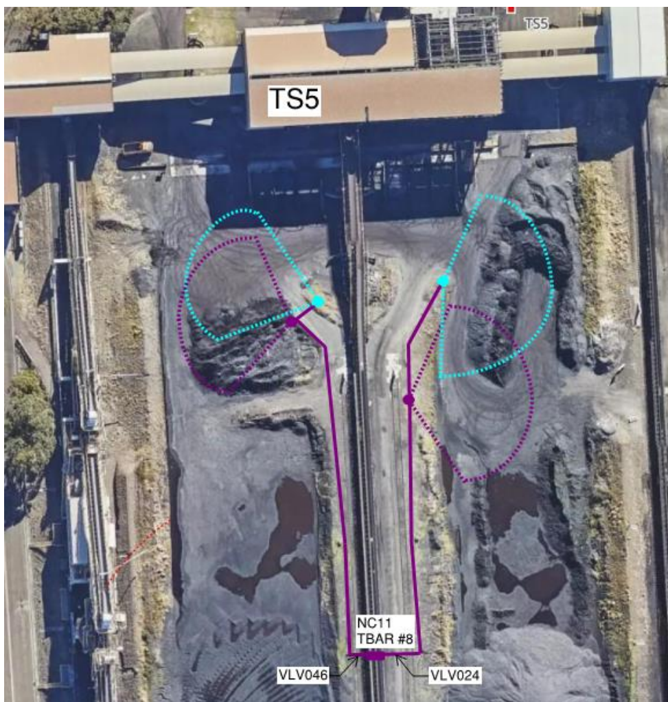
Figure 19: Capital Project to install new spray guns at north end of stockyard
