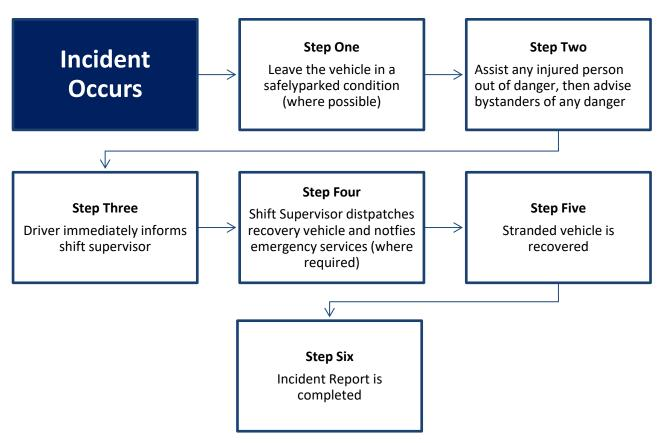
To ensure quick response, all incidents must be reported immediately to your shift supervisor. For incidents on the public road network contact emergency services and TfNSW as required and others if support is needed. For incidents at the mine site and PKCT, the site controller shall be contacted (i.e. mine site or PKCT as appropriate).
