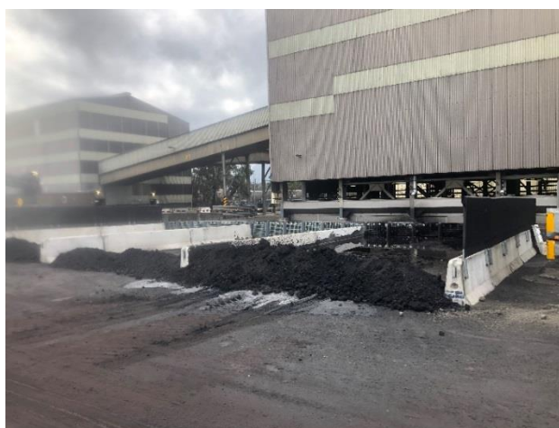
Figure 19: Spillage coal drying pits speed up the drying process and minimises coal handling to improve dust control.
